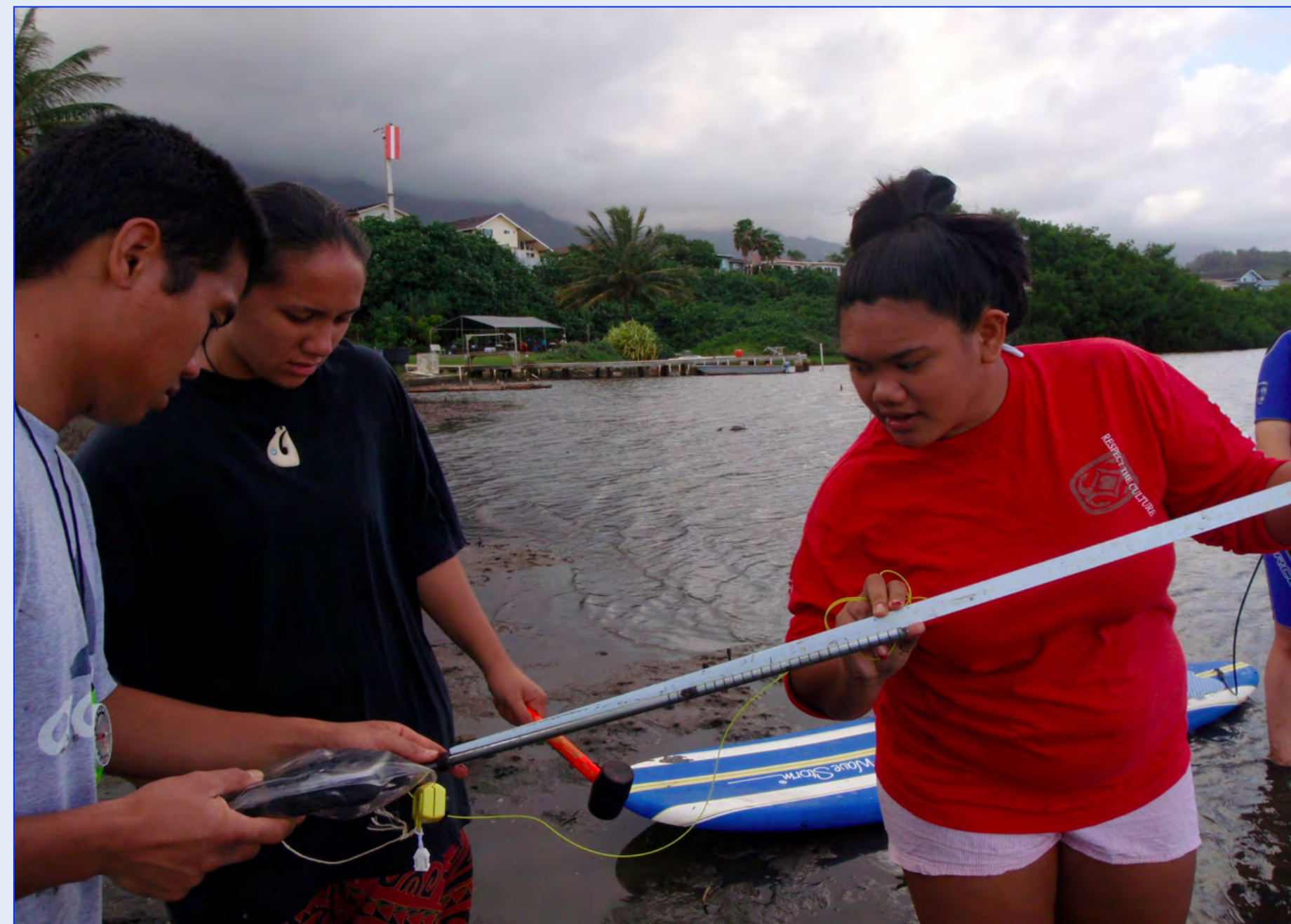
Measuring sediment depth in the fishpond
